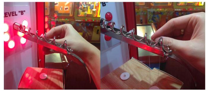
4. After placing prizes reach the locking pin over hanging ties supporting prizes and screw the locking pin into the prize arm by turning it in anti-clockwise direction.
