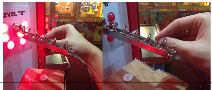
4. After placing prizes reach the locking pin over hanging ties supporting prizes and screw the locking pin into the prize arm by turning it in anti-clockwise direction.
