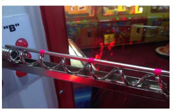
3. Put prizes on appropriate loops, starting from this one, which should fall on the end. Remember that the first prize should be placed on the first loop of the spiral, marked by colorful sticker, counting from the beginning, and the next have to be placed two loops further – exactly in spaces marked by colorful stickers.
